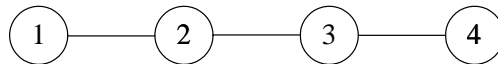
Figure 7.1. The graph representing the Markov chain X_1 \rightarrow X_2 \rightarrow X_3 \rightarrow X_4 .
